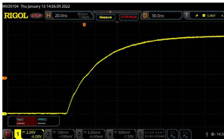
Figure 4: MOSFET Gate Voltage
