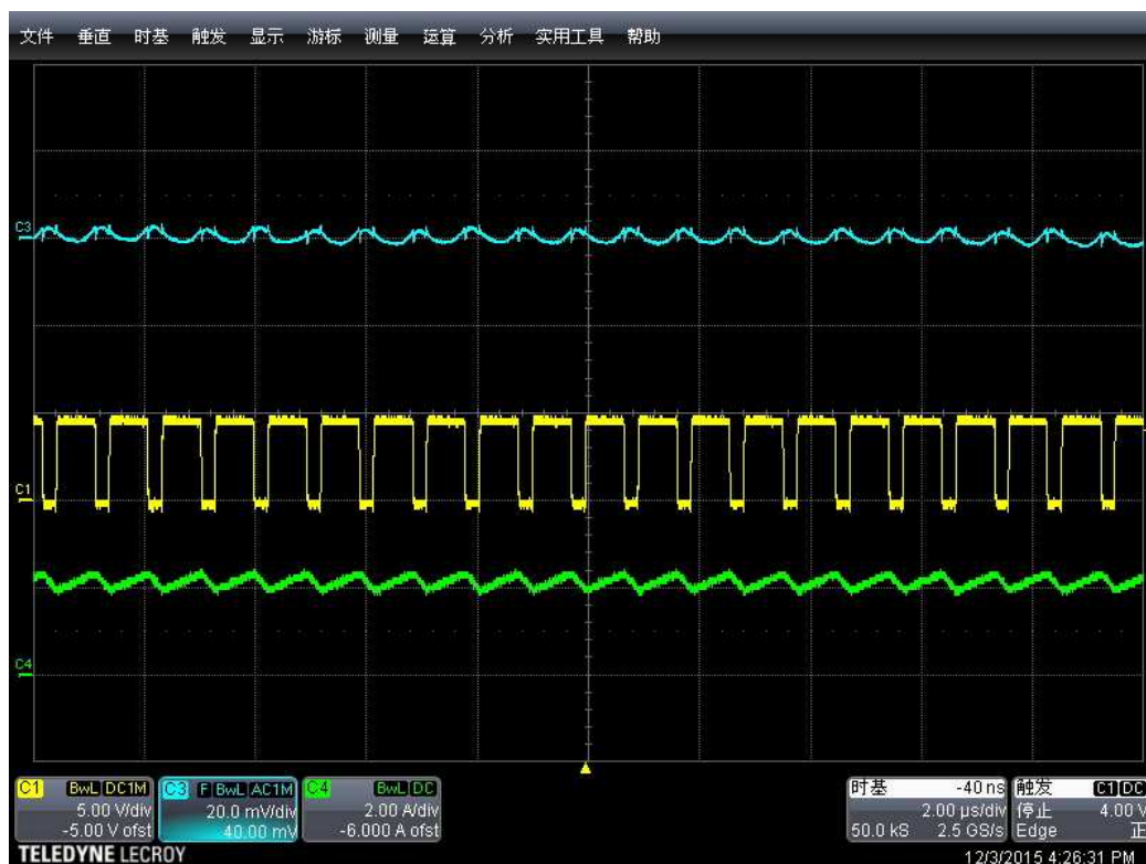
Operation waveform at Iout=2A (Blue-VoutAC; Yellow-Vsw; Green-IL)
