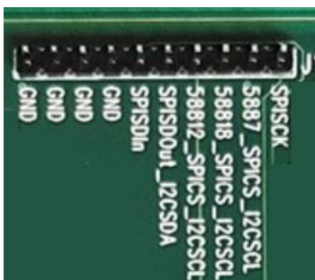
Figure 3: Box #5 - External I2C/SPI Connector Pinout
