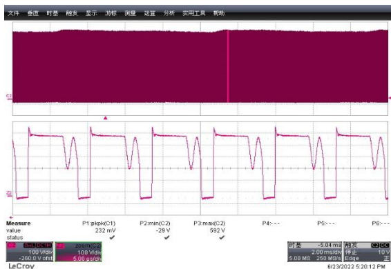
Figure 16: Q1 Vds Voltage stress
