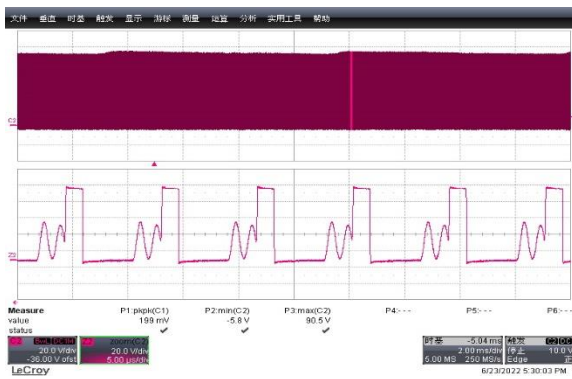
Figure 17: Q2 Vds Voltage stress
