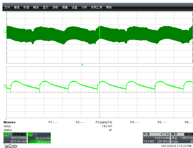
Figure 27: 90Vac/60Hz 20V/2.25A \Delta V=142\text{mV}
