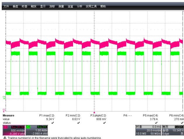
Figure 31: VIN=90VAC, 9V @ 0.4 ~ 3.6A
