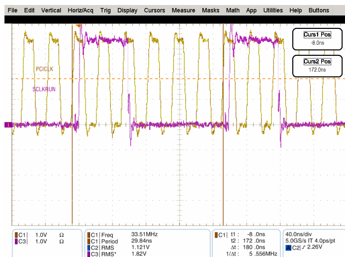
Figure 2: Tcrrep for S_CLKRUN#
